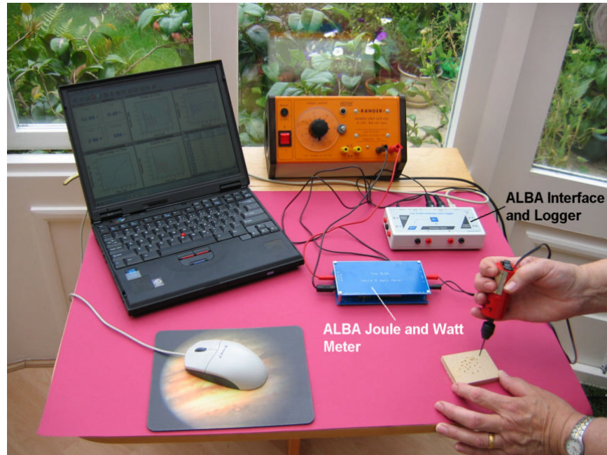
Figure 1 Investigating a drill on/off load with the ALBA Joule and Watt Meter
